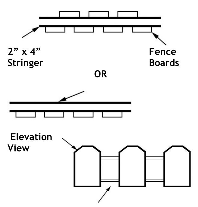
2 inch Minimum Spacing Between Fence Boards
